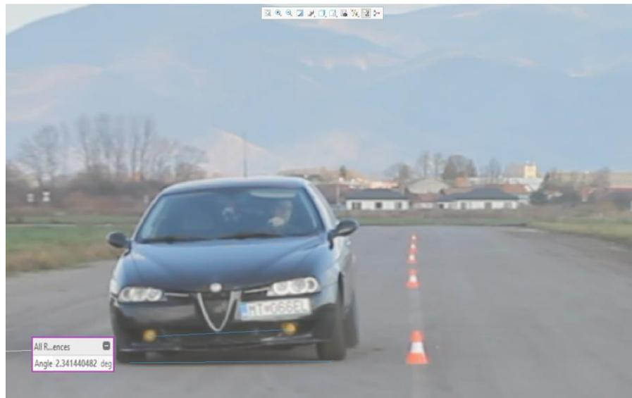
**Fig. 6. Vehicle body roll angle measurement in Creo Parametric 4.0 computer program**
